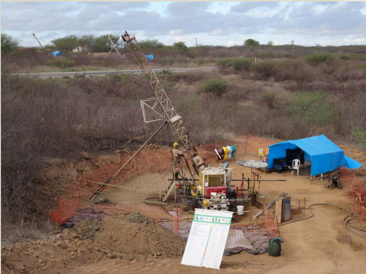
Figure 1; Three diamond drill rigs operating near the highway at Borborema, 14 February 2012.
