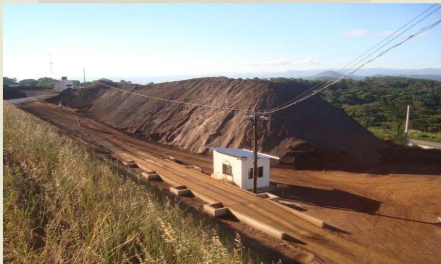
Figure 3: Stockpiled fines on site – Posse Iron Ore Mine, May 2013. (50% Fe <6mm material)
