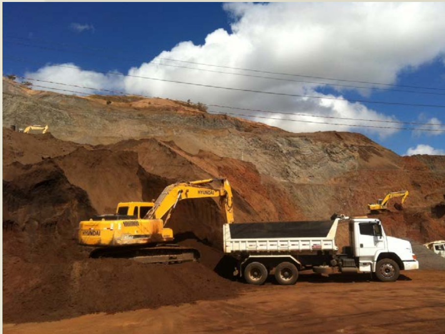
Figure 5: Free digging at Posse Mine
