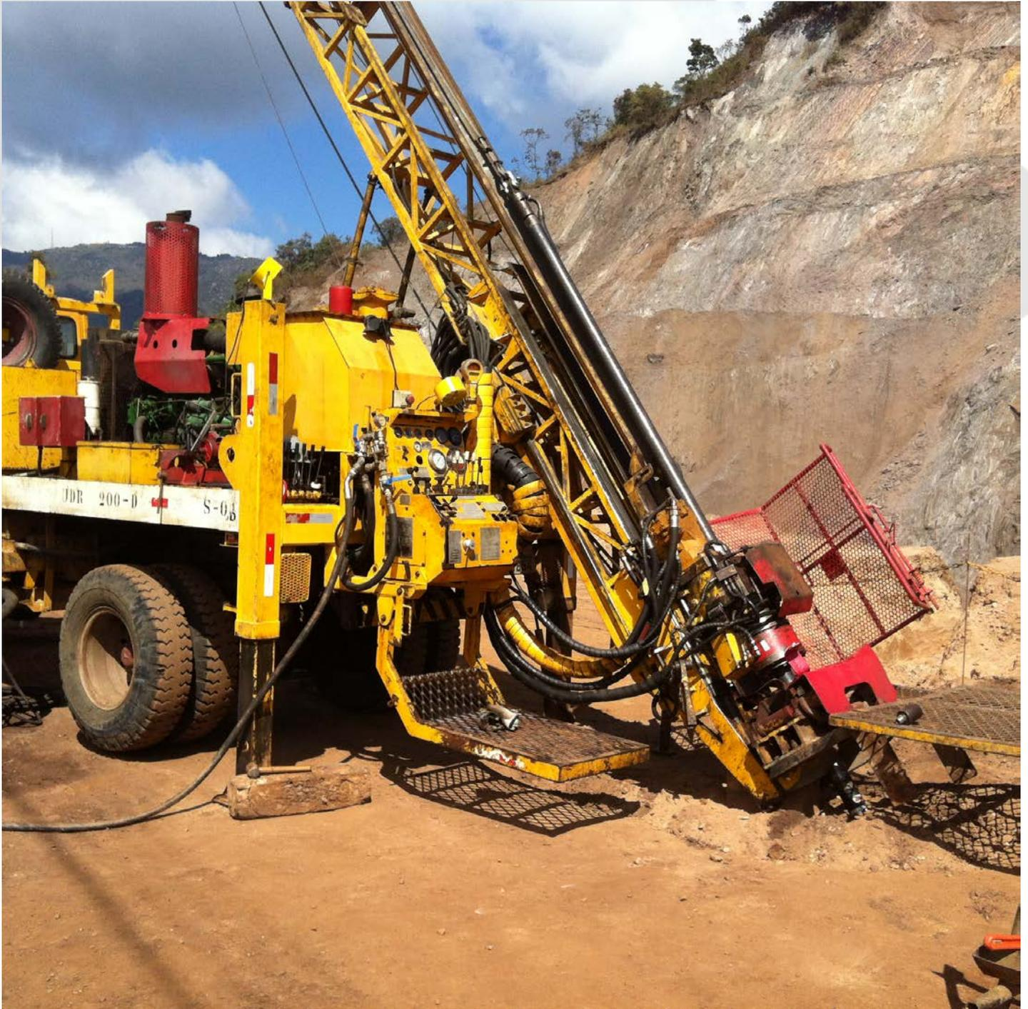
Figure 1; Diamond drilling underway at Posse Iron Ore Mine
