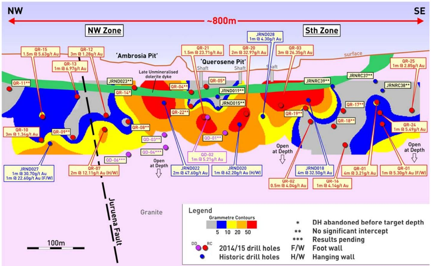
Figure 3: Querosene long section with gold gram x metre contours
