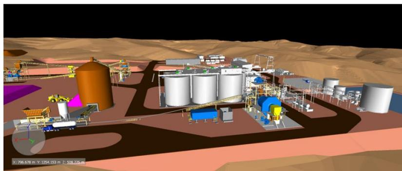
Figure 5. View to the south of the revised Borborema plant layout, showing grinding circuit, CLIL tanks and fine ore bin/emergency stockpile feeder to the left
