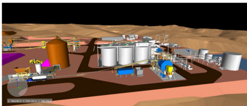
Figure 5. View to the south of the revised Borborema plant layout, showing grinding circuit, CIL tanks and fine ore bin/emergency stockpile feeder to the left
