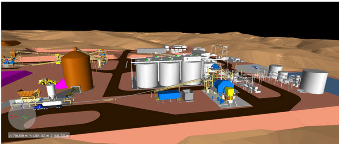
Figure 3. View to the south of the Borborema plant layout, showing grinding circuit, CIL tanks and fine ore bin/emergency stockpile feeder to the left
