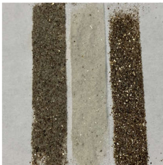
Figure 1. Picture showing the gold plant leach residue (left), non magnetic reject (centre) and mica rich magnetic concentrate (right)
