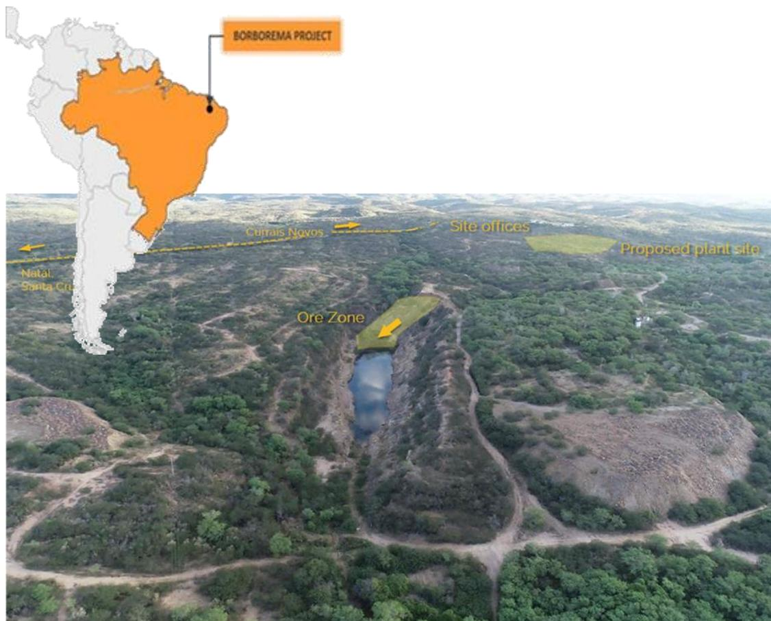
Figure 1. View to the south west over the Borborema pit showing the exposed ore zone and infrastructure.
