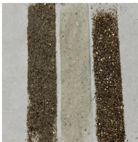
Figure 2. Picture showing the gold plant leach residue (left), non magnetic reject (centre) and mica rich magnetic concentrate (right)
